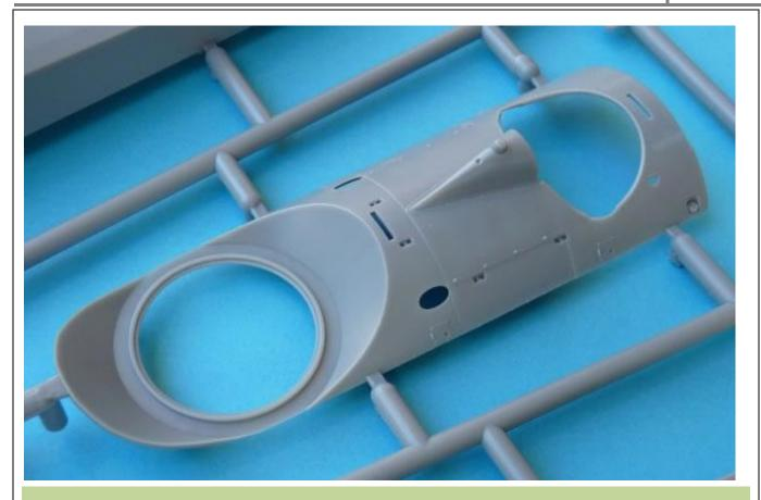
Once the fuselage halves are together it's time to add the cockpit coaming. It's a clever piece of moulding and the design ensures a better fit than would have been the case with multiple parts. The only compromise is that the sprue gate falls close to a couple of rivets that will have to be replaced after the clean-up process.
